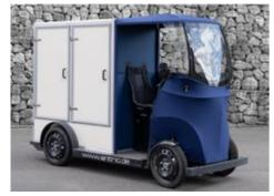
Antric has designed and engineered the Antric One, an auto-grade four-wheeled e-cargo bike that has been successfully piloted in Europe. The Antric One is purpose-built for delivery services and general cargo transport.
